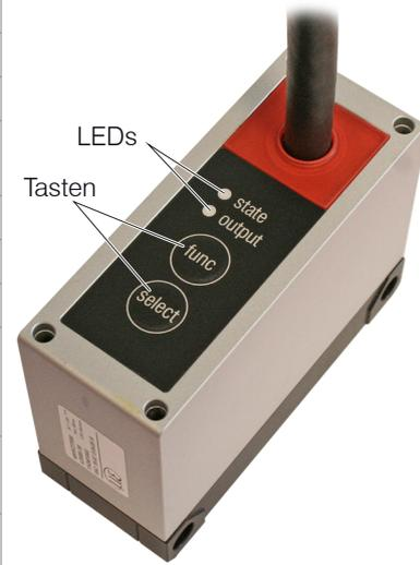
Tab. 3.1: LEDs am Empfänger (Receiver)
