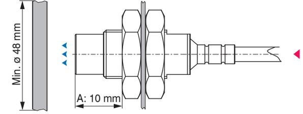
Montage, Abmessungen in mm
