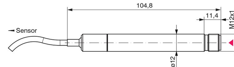
DT3005-x, Abmessungen in mm
